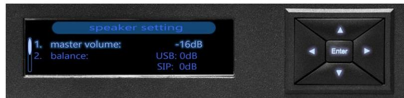
Use the speaker setting to control the maximum output level transmitted to loudspeakers via the master volume. Also use this option to balance the level of USB, SIP or analog audio inputs.
