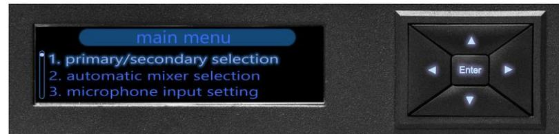
Use this option to identify and select primary and secondary MT700 Stingray Mixer(s) connected in a daisy chain. A primary mixer is the unit connected directly to your intended communication mode – SIP, USB, or analog, for example. Designating a daisy-chain primary mixer automatically opens its connection to your intended communication mode and applies all primary settings to the secondary units that follow. When you
