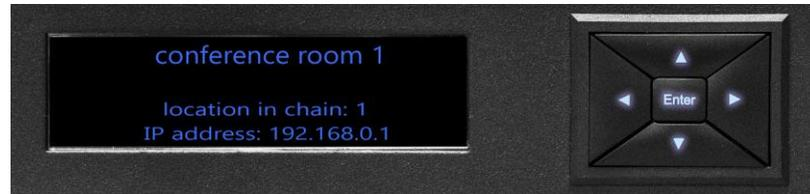
To configure the MT700 Stingray Mixer, select from the seven options on the menu-access screen. When ready to make a selection, press either the center [ENTER] keypad button, or the keypad's rightward directional [>] or downward directional [v] button. To return to a previous screen press the leftward directional [<] or upward directional [^] button.
